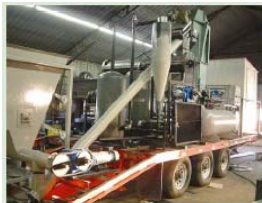
← A small-scale portable reactor for liquid fuel production by distributed fast pyrolysis
